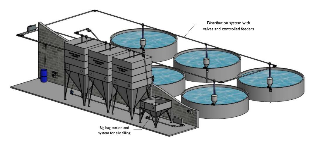
Complete feeding system that handles feeding procedure from feed reception to dosing from feeders. The feeding system has two circuits. One circuit receives feed and filling silos. The other circuit distributes feed to the feeders and subsequently reallocates feed from feeders to fish.
