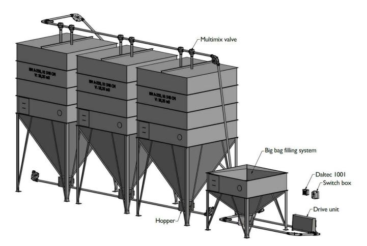
The filling system is used to fill the silos from a big bag filling station. The filling is quite simple: select via controls, the silo to be filled, hang a big bag over the filling station and start the system.
